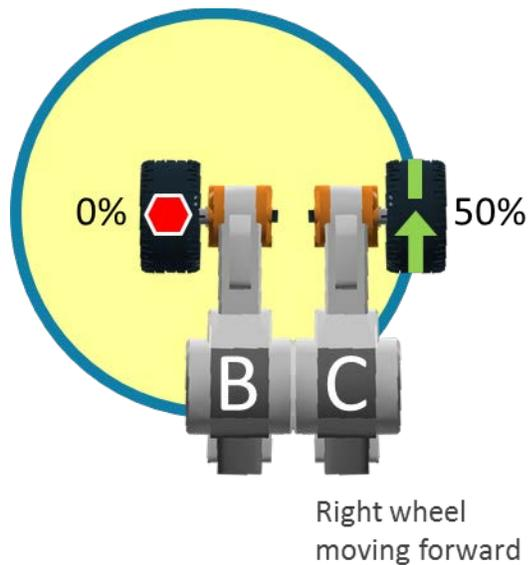
1. Program the robot to turn complete a left 90% turn using the motors speed shown.
