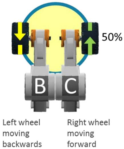
1. Program the robot to turn complete a left 90% turn using the motors speed shown.
