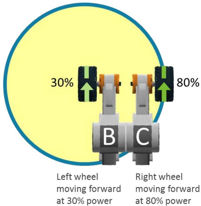
1. Program the robot to turn complete a left 90% turn using the motors speed shown.
